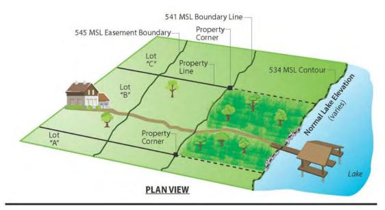
Figure 4-4. Projected Side Yard Lines and Hard Erosion Control BMP Installation
